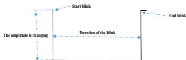
Figure 5. The proposed amplitude blink gesture
