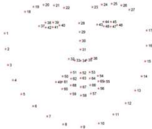
Figure 2. Visual representation of 68 facial landmark points
